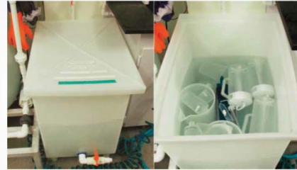
Figure 3. Opaque bin used to hold the 1.98% bleach disinfection solution. The lid was kept on the bin when not in active use, to decrease light exposure and minimize evaporation.
